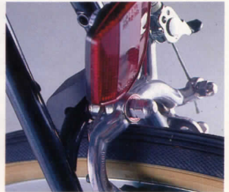
Curved, reinforced brake bridge
