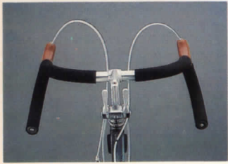
Randonneur style alloy handlebars with cushion grips and extension levers
