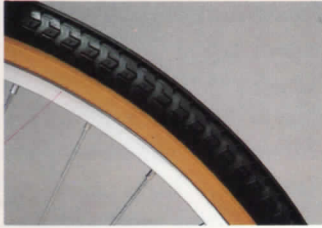
650 x 35C wheels with alloy rims and Raleigh's high center ridge, multi-pressure tires
